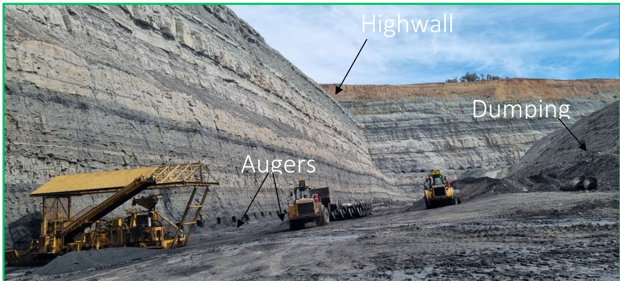
Figure 2: View of coal exposure and structures exposed in the highwall in A South.
