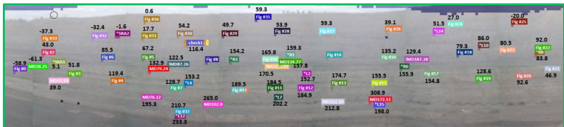
Figure 22 Ground-based radar monitoring highwall displacement trends (Dec 2022 – April 2023) in A Pit Highwall.
